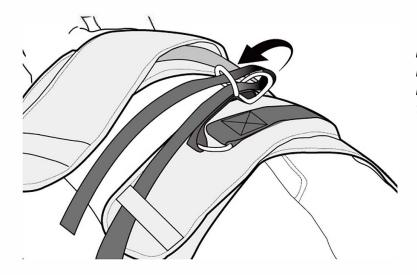
BRING the open end over the second ring then INSERT through the first ring. PULL the open end to increase tension.
